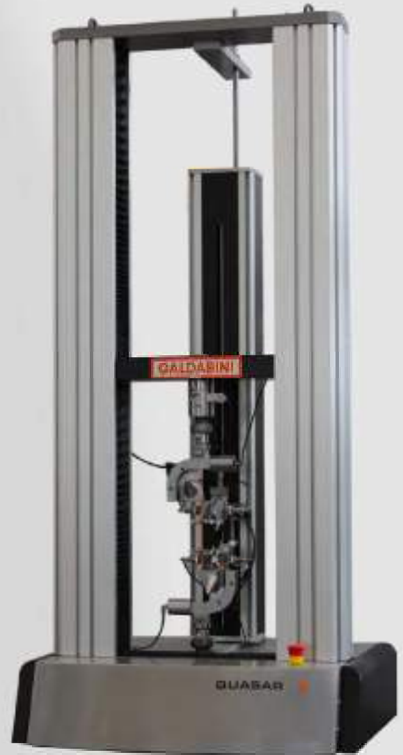
Universal testing machine Quasar 5 with Micron extensometer
